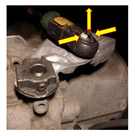
6. Using the supplied pin removal tool, align the bolt of the tool with the pin and wind the bolt with a 10mm socket and ratchet to push the pin out the back of the shifter shaft, then unwind the bolt out towards you so you are able to remove the pin removal tool. Pull the OE shifter upwards to remove it.
